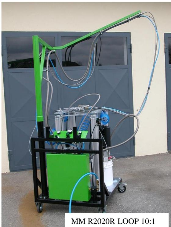
This technical data sheet is valid for all MM R2020R, MM R20020R and MM R200200R continuous bulk dispensing equipment, manufactured by Mayer & Mayer HandelsgmbH, Gewerbeweg 16, 7411 Markt Allhau, for dosing of EBS Acralock structural adhesives, ratio 10:1 and 1:1, out of standard straight headed 20 l pails or 200 l drums.
