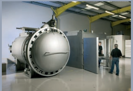
The Basingstoke composites facility includes full laminating, trim and autoclave capability
