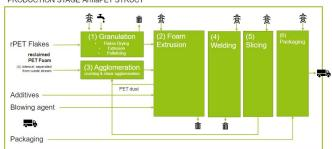
Obtained recycled PET granules are further processed into foam through foaming extrusion, in the presence of halogenfree
