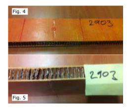
is marked. Note the **permanent deformation and damage to the skin**. Figure 5 shows typical **buckling damage** to the honeycomb core cell walls under the impact location.
