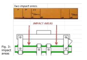
in the core when testing in 4-point bending mode, see fig. 3. The beams were tested for two different boundary conditions. At first the beams were fully supported on the back side when impacted, resting on a stiff aluminum profile.
