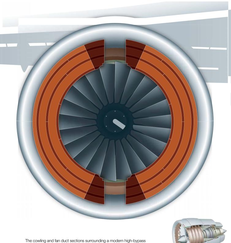
The cowling and fan duct sections surrounding a modern high-bypass airplane turbine engine are collectively referred to as the nacelle. The center image shows a nacelle cowl assembly. Honeycomb is used throughout the nacelle's construction, providing support that withstands vibration, high temperatures and offers sound attenuation.
