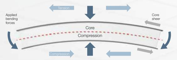
A sandwich structure consists of two relatively thin, yet strong and stiff, skins or facings on both sides of a thick, yet lightweight, core material. The skins take up the normal stresses in-plane and give the structure a hard-wearing surface. The core material absorbs the shear forces generated by out of plane loads, distributing between the skins and spreading them over a
