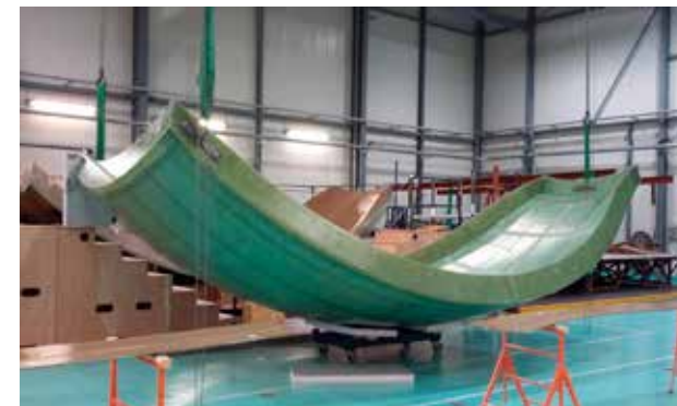
©Multiplast: panels cored with ArmaPET Struct GR80 in 50 mm
