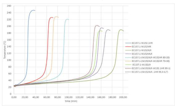
With HR label is identified the high reactivity hardener W152.1HR, generally suitable for small dimensions repairing or as reactivity modifier for other hardeners. The mixture of W152XLR with W152.1HR in different ratios allows to obtain intermediate reactivities. The systems are approved by DNV GL.
