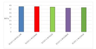
The composite laminates has been obtained by infusion of a  $600g/m^2$  glass E tissue. From laminating of 5 mm of thickness cured at room temperature and stabilized at 50°C for 16 hrs were obtained specimens following ASTM D2344 code.
