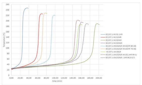
With HR label is identified the high reactivity hardener W152.1HR, generally suitable for small dimensions repairing or as reactivity modifier for other hardeners. The mixture of W152XLR with W152.1HR in different ratios allows to obtain intermediate reactivities.
