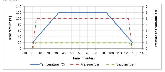
HexPly® M10R is a flexible curing system and can be cured at temperatures from 85 to 150°C, at pressure between 0.9 to 5 bar. Heat up rate can be also adapted (from 0.5 up to 10°C/min) depending the part design.
