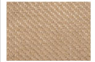
ampliTex<sup>™</sup> is a range of natural fibre reinforcement for composites, engineered to offer very high performance at low weight, with minimal impact on the environment.
